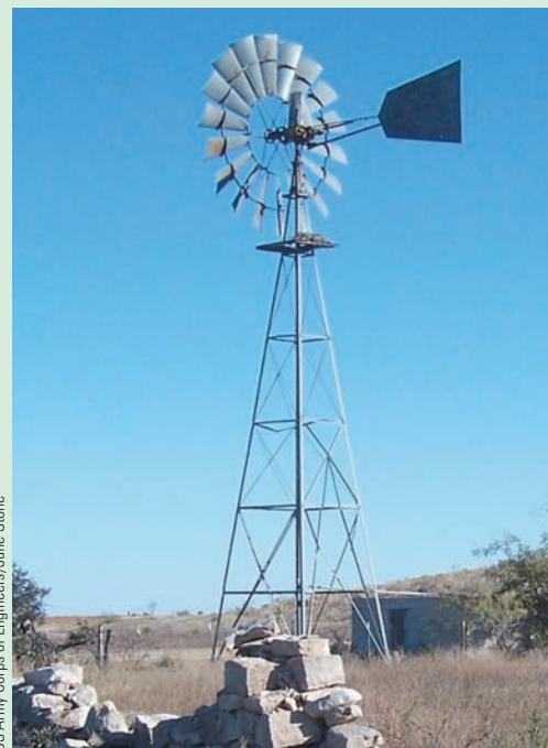
Windmills like this, used to pump well water on ranches and farms, are in semiarid and arid regions of North America.
